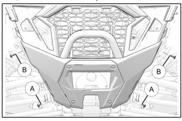
2. Remove bumper fascia from vehicle and carefully set aside.
