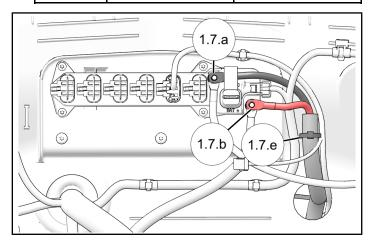
10. Do not remove existing nuts from NEGATIVE and POSITIVE terminals. Secure harness with two nuts (8).
