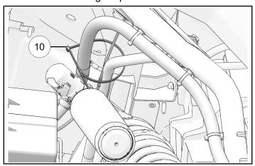
5. Route winch harness over suspension and position contactor box on firewall. Install two outside screws ⑥, until tight, to automatically align inside mounting location.
