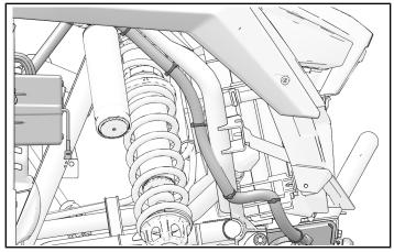
2. Secure to chassis with edge clip and push-pin clip.
