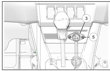
3. Join remote socket connector ③ to winch remote connector 1.17.d.
