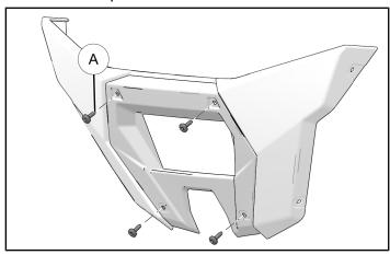
2. Install new winch cover ④ with four retained bumper fascia fasteners ④.
