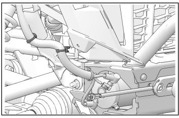
3. Secure to chassis with three push-pin clips.
