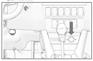
2. Install winch remote socket ③ with two remote socket fasteners ⑤ until tight.
