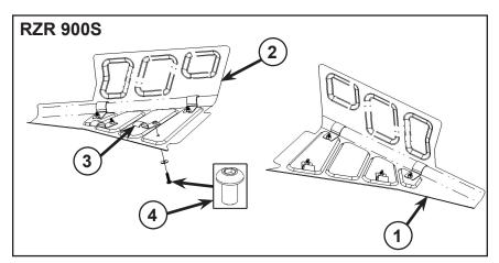
4. Install the LH and RH A-Arm guards (1; 2) on the A-Arms (C). Tighten the screws to 8 ft. lbs. (10.5 Nm) as shown in figures.
