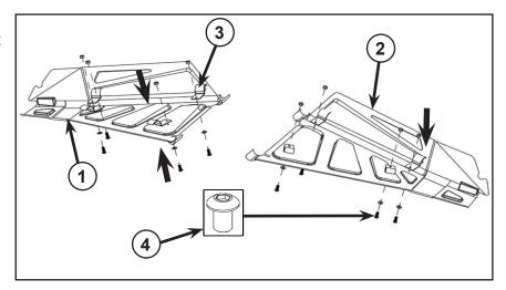
4. Install the LH and RH A-Arm guards (1; 2) on the A-Arms (C). Tighten the screws to 8 ft. lbs. (10.5 Nm) as shown in figure.
