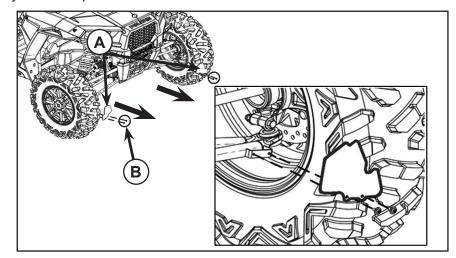
3. Install the clamps loosely on the LH and RH A-Arm guards (1; 2) using boot clamps (3) and screws (4) as shown in figure.
