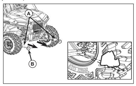
3. Install the clamps loosely on the LH and RH A-Arm guards (1; 2) using boot clamps (3) and screws (4) as shown in figures.
