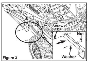
5. Attach the M6 screw, M6 washer and M6 nut. Figure 4.
