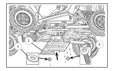
6. Remove LH rocker panel (D) by removing fasteners (E) (six plastic push pins and five screws). Retain fasteners.
