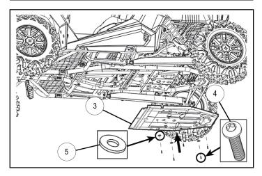
5. Loosely install middle skid plate ② using five each screws ④ and cup washers ⑤.
