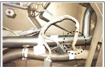
d. Position amp ® (with pre-attached inner bracket) on inboard side of chassis tubing. Install lower tabs in outer bracket ⑨ to mating slots in inner bracket. Rotate outer bracket upwards, then secure both brackets to chassis tubing using two screws ⑩.
