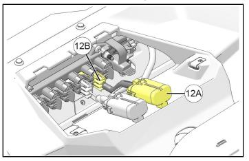
b. Open power cap on vehicle terminal block at any open location, then plug in connector 12B (identified as: **ACC 12V**).
