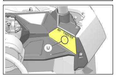
e. Remove template, then carefully drill harness passage hole at marked location using 1.5 inch (38 mm) hole saw.
