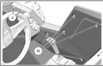
e. From outside of vehicle, and while supporting exterior body panel, remove final two screws
