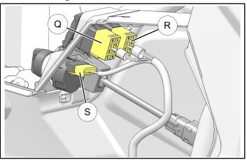
c. Reroute chassis breakout harness from INSIDE of chassis tubing to OUTSIDE of chassis tubing as shown.
