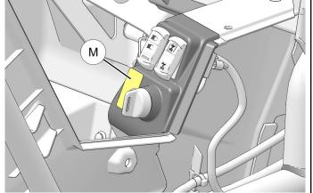
b. Install Bluetooth<sup>®</sup> controller <sup>(1)</sup> into switch cutout. Ensure volume markings are up, and auxiliary input jack is down.
