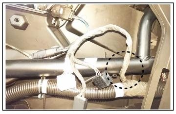
d. Position amp (a) (with pre-attached inner bracket) on inboard side of chassis tubing. Install lower tabs in outer bracket (b) to mating slots in inner bracket. Rotate outer bracket upwards, then secure both brackets to chassis tubing using two screws (10).
