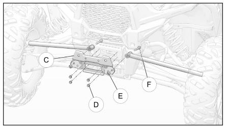
Fasten bracket bumper support (3) on to the front suspension mount bracket by hand tighten M10 screws (9) and M10 nuts (12).
