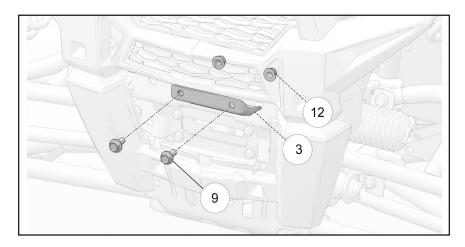
Mount bracket bumper support (3) on to the fairlead mount bracket by fastening plate weldment (4) and two M10 screws (9). Torque to 40 ft. lbs. (54.2 Nm).
