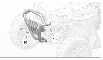
14. Fasten two M10 screws (11) on the weld front bumper as shown in figure. Torque top and bottom screws to 40 ft. lbs. (54.2 Nm).
