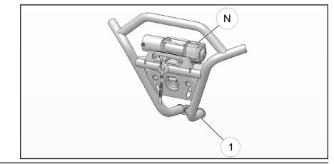
12. Align the weld front bumper (1) to the holes of the front suspension mount bracket (C) on the vehicle frame as shown in figure.
