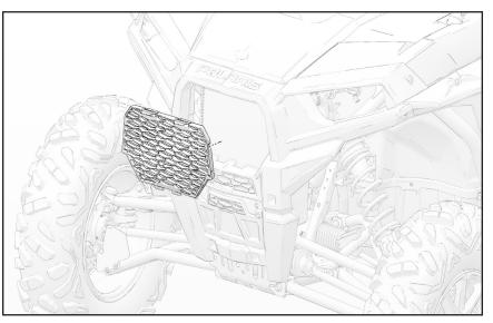
Remove winch cover (A) by removing two screws (B) as shown in figure. Keep winch cover and screws for reuse.
