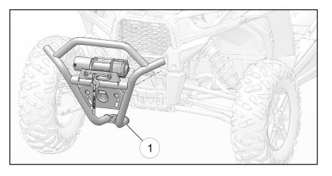
13. Loosely install weld front bumper by fastening two M12 screws (10) and relevant nuts (13) as shown in figure.
