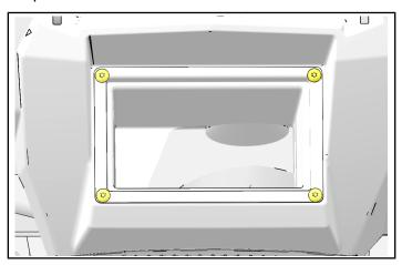
22. Locate upper instrument panel. Lay template on upper instrument panel and cut panel along dotted line for installing defrost vent ②. (Use Template 5, attached at end of instructions).
