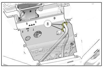
12. Place coolant clamps on coolant return hose as shown. Cut hose between clamps. Remove 1" of hose from one of ends to make room for thermostat assembly. Install thermostat assembly
