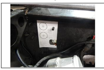
7. Locate bracket mount template. Position template on inside of firewall as shown (Use Template 2, attached at end of instructions). Repeat marking process described in previous Step. From inside of firewall drill out holes using a 3/8" drill bit.
