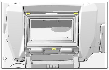
21. If your storage compartment does NOT have flip down front lid do following.Drill 3/16" holes in each corner of storage box.Insert storage box and secure with screws provided.
