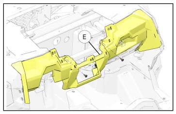
6. Locate firewall hose template. Position template on inside of firewall as shown (Use Template 1, attached at end of instructions). Mark center of each hole using a sharp punch or awl. From inside of firewall drill holes using a 1 3/8" hole saw.
