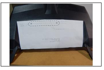
23. Cut out one of accessory knock outs in upper instrument panel to mount heater control switch
