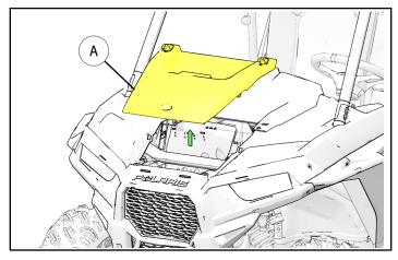
3. Remove upper instrument panel (B) by removing two screws and disconnecting ignition, headlight switch, accessory plug, AWD switch, and any other accessory controls that may have been added.
