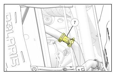
15. Install top hose (5) from heater core to small part of "Y" fitting (7) as shown and tighten clamp. System is now closed and all coolant clamps can be removed.
