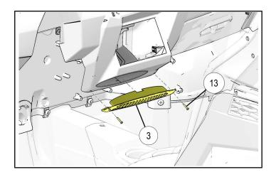
17. Secure center storage compartment (1) cap to back of heater assembly using fastener provided as shown.
