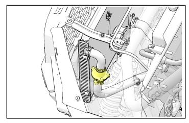
13. Install bottom hose ④ from heater core onto thermostat assembly ⑥ and secure with a hose clamp. Install a coolant clamp onto lower heater hose near thermostat assembly before removing coolant clamps above and below thermostat assembly.
