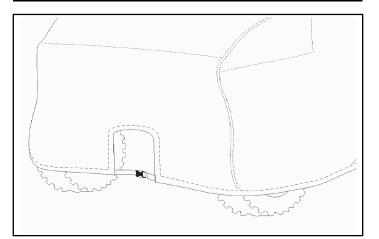
4. Thread strap through rear center loop. Insert strap into partially closed ratchet and begin to operate ratchet mechanism.
