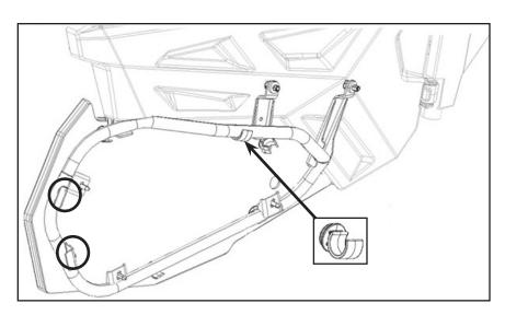
11. Press the liner to the door frame until the four plastic clamps (3) fits snug inside the frame. See figure.
