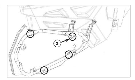
12. Reinstall the screw (A) removed in Step 8 and attach door liner (1) to hinge bracket. Tighten screw to torque of 16 ft. lbs. (21.8 Nm). See figure.
