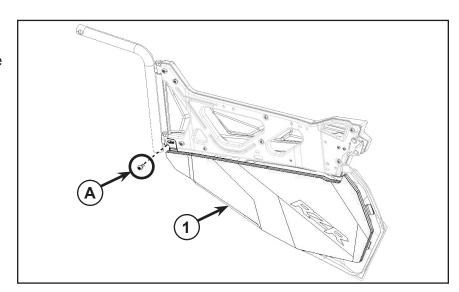
13. Repeat Steps 8-12 on the passenger side to install RH lower door liner (2).
