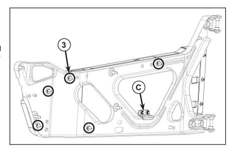
7. Reinstall the two M8 screws (A) removed in Step 2 and attach the door liner on to the door hinge brackets as shown in figure. Tighten screws to torque of 16 ft. lbs. (21.8 Nm).
