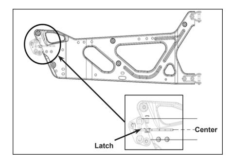
8. Repeat Steps 2-6 on the passenger side to install RH upper door liner (2).
