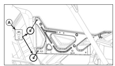
4. Align the LH door liner (1) to the upper door (B) assembly. See figure.
