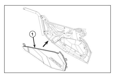
10. Slide the two rear clamps onto the frame rearwards. Ensure the rear upper 90 degree clamp must be snap to the frame by pivoting the liner, once the two rear clamps are in place. See figure.
