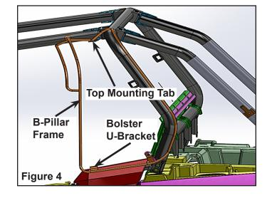
2. Install the mounting bracket using the top ROPS bolt at the bottom of the B-pillar. Figure 3.
