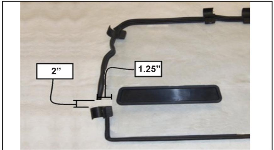
4. Install the ROPS attachment bracket to the C-Pillar, using a hose clamp, as show. The hinge of the bracket should face the outside of the vehicle. The hose clamp should seat directly beneath the horizontal ROPS bar. This should be finger-tight only; they will be adjusted during a later step.
