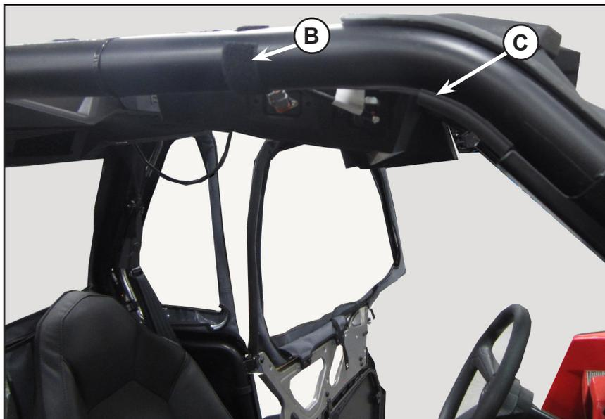
14. Roll up all windows, and close all zippers. Adjust all hook and loop fasteners on the fabric doors and door frames to tighten the fabric on the frames. The fabric can be relaxed or pulled tighter to adjust the positions of the seals around the door. When finished, the doors should have a tight seal with the vehicle.
