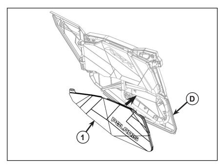
3. Press the liner to the door frame (E) until the four plastic clips (3) and 90° plastic clip (4) fits snug inside the frame as shown in figure.
