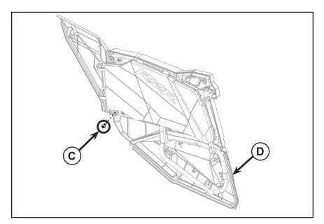
2. Align the LH door liner (1) to the rear lower door (D) assembly as shown in figure.
