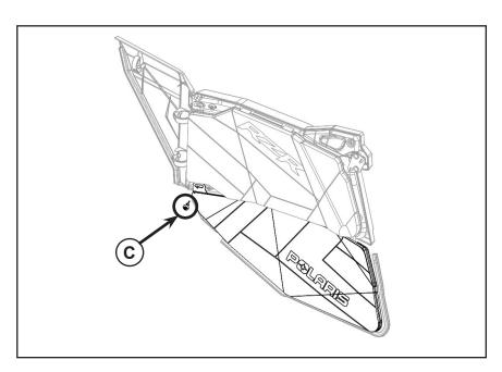
5. Repeat Steps 1-4 on the passenger side to install RH lower door liner (2).
