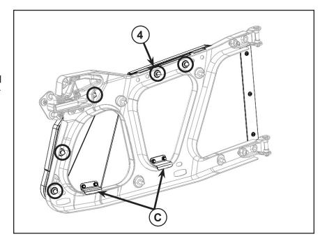
7. Install the two M8 screws (3) provided in the kit and attach the door liner on to the door hinge brackets. Tighten screws to a torque of 16 ft. lbs. (21.7 Nm) as shown in figure.
