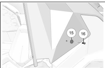
4. Hook Z-clip ② onto rear body plastic and align with previously installed fastener. Secure with one nut
