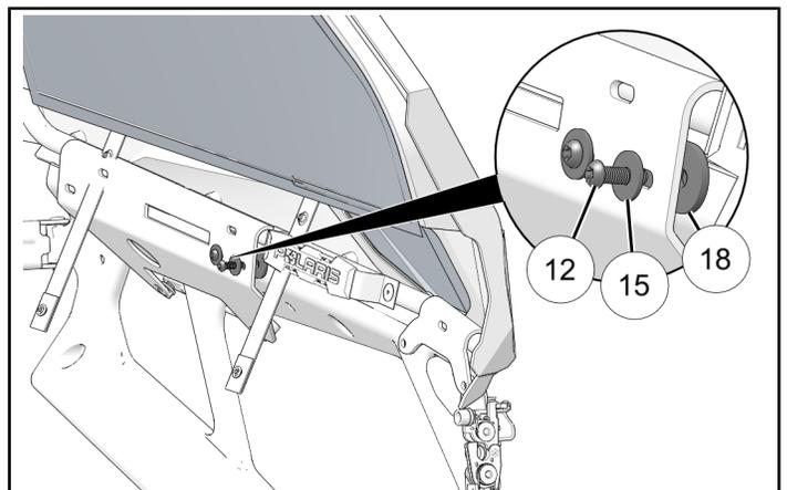
4. Put one door bracket fastener ⑫ through one washer ⑮, one spacer ⑲, and door frame.
