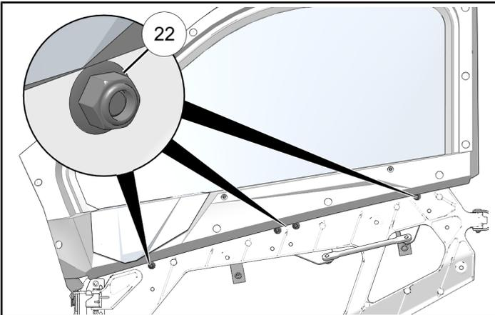
9. Counter-hold nuts ⑳ (where applicable) and torque five fasteners ⑫ to specification
