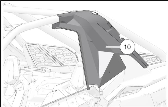
2. Attach rear shroud to roll cage with three hook-and-loops straps ⑭.
