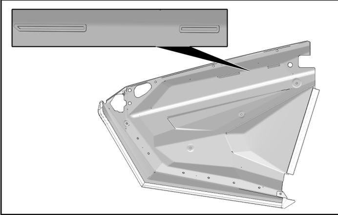
2. Drill one **1/4 in (6.5 mm)** hole at each end of rectangular embossed lines. Cut remaining plastic, between drilled holes, with utility knife or equivalent.
