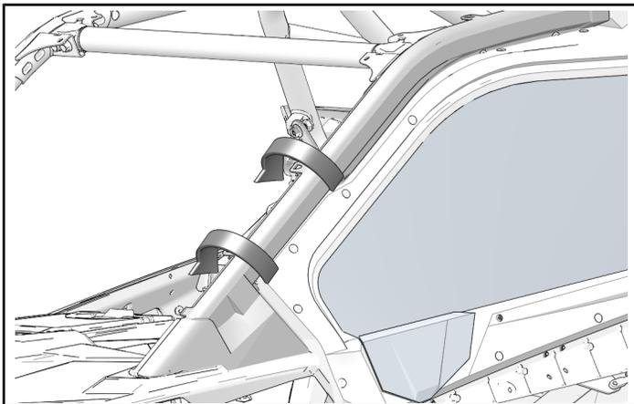
3. Counter-hold nuts ② and torque shroud fasteners ⑩ to specification.
