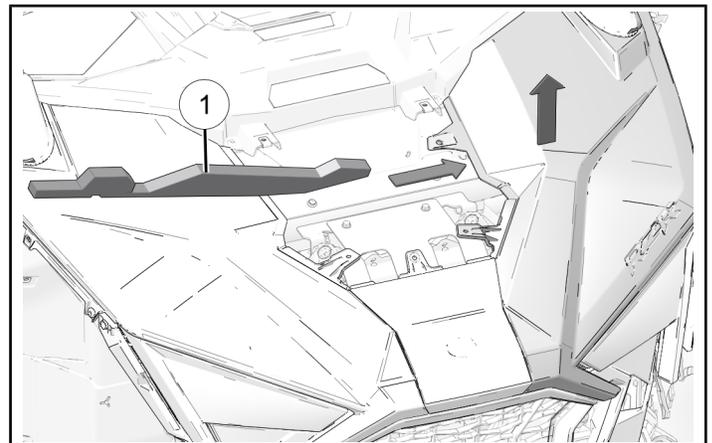
3. Lift upper fender upwards and slide hood seal ② under panel along chassis tube.
