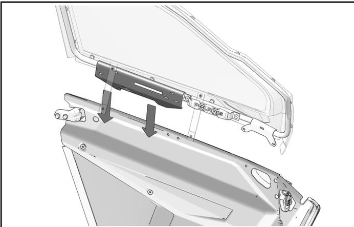
4. Secure door bracket fasteners with four nuts (22).
