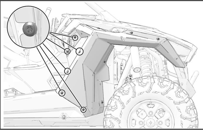
3. Install the most front fastener (shorter) and one push-pin rivet.
