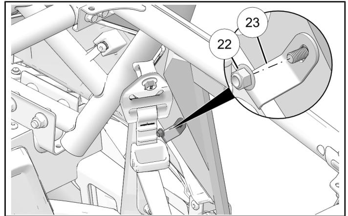
5. Counter-hold nut ㉒ and torque fastener ⑯ to specification.
