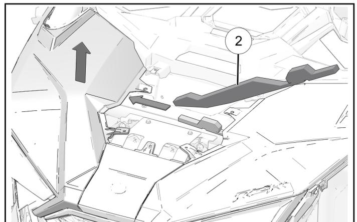
4. Reinstall two fasteners and two push-pin rivets. Torque two fasteners to specification.
