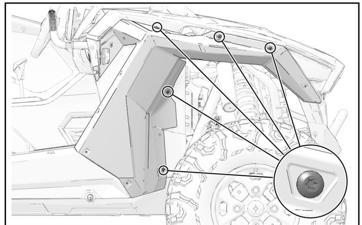
2. Install six fasteners at rear of front fender.
