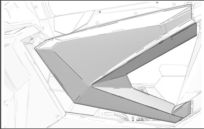
2. From inside of door, install door panel with eleven door panel fasteners.
