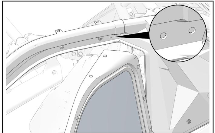
2. Install front shroud to rear shroud with two fasteners ⑩, two washers ⑮, and two nuts ②.
