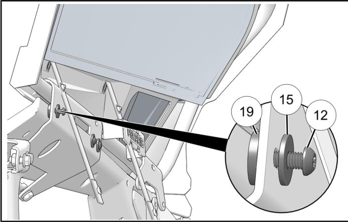
7. Install front-most part of door panel with one fastener ⑫ and one washer ⑮.
