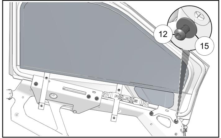
5. Put one door bracket fastener ⑫ through one washer ⑮, one spacer ⑲, and door frame.
