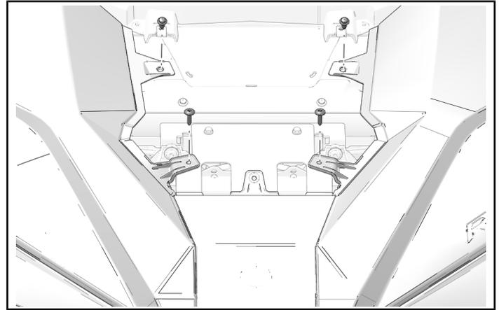
2. Lift upper fender upwards and slide hood seal ① under panel along chassis tube.
