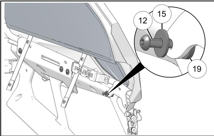
8. Move door assembly to most-rearward position, making sure door seals firmly against front and rear shroud.
