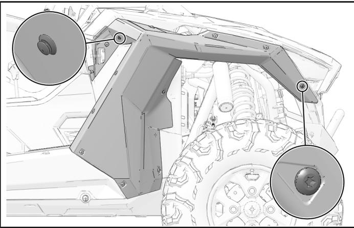
4. Torque all fender fasteners to specification.
