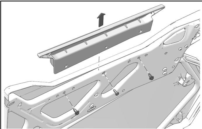
2. Remove and keep eight door fasteners to remove door from door frame.
