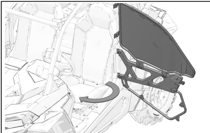
2. Torque clamp fasteners ⑫ to specification.
