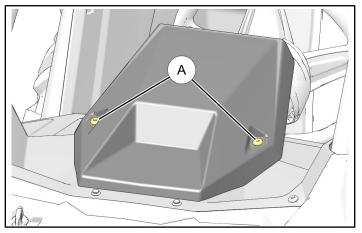
b. Remove RH A-pillar access cover ® by grasping rear inboard corner of cover with fingers, then lift to detach three locking tabs ©, two posts ®, and two locking tabs €. Set cover aside.
