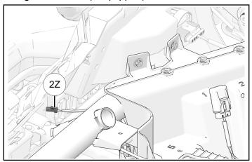
11. Route audio harness to passenger side. Secure to front cab panel with routing clips.
