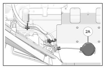
16. Route Ride Command® harness down along radiator shroud. Install with routing clips. Join air temperature gauge ⑨ to connector 2X and install onto radiator shroud.
