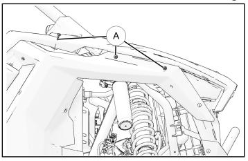
3. Remove and retain two hood fasteners (A) and one push-pin rivet (B).
