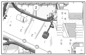
2. Install fuse holder 2T onto accessory mounting panel. Secure harness to accessory mounting panel with one routing edge clip.
