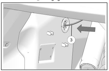
3. Route antenna harness ③ along accessory mounting panel. Secure in tabs along edge.
