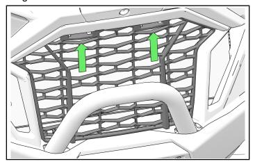
2. Tip grille forward and pull out until bottom tabs are clear of front fascia and bull bumper.
