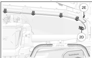
12. Join audio harness connector 2E to tweeter and connector 2D to driver.
