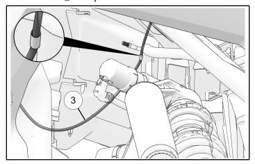
2. Pass harness 3 through grommet in firewall.
