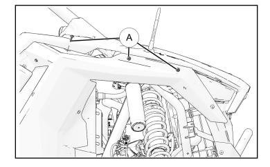
3. Reinstall hood nose panel with one fastener (A).
