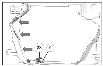
17. Carefully pull up on right-hand hood panel and install V2V antenna (1) onto vehicle.
