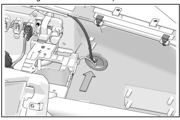
14. Secure audio harness to electrical chassis harness with three attached cable ties. Secure antenna harness with at least one attached cable tie.
