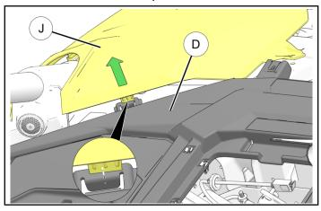
6. Carefully lift edge of right front fender (®) to release tab from dashboard top (®) as shown.
