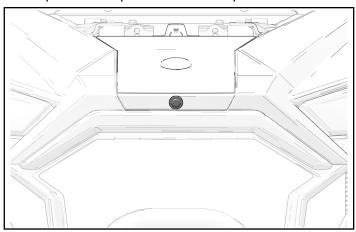
3. Join camera connector to chassis harness connector.
