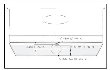
6. Drill out center hole with 13/16 in. hole saw.
