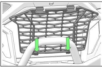
2. Push top of grille into front fascia until two tabs engage with fascia and are secure.
