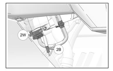
5. Route audio harness to driver side. Secure to front cab panel with routing clips.
