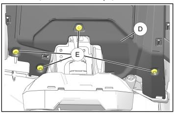
4. On front of vehicle, near rear edge of center hood panel opening, remove and retain two screws © from dashboard top ①. Remove and retain two pushpin rivets ① from front side panels.
