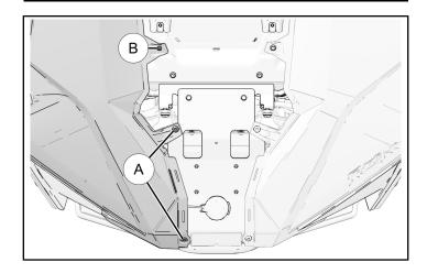
2. Reinstall right-hand hood panel with three hood fasteners (a).
