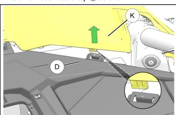
7. Carefully keep panels ① and ⑥ up and away from tabs and remove dashboard top ⑩ by tilting rear section up and pulling out toward rear.
