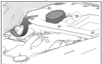
18. Secure V2V antenna (10) with slip-nut (15). Join V2V antenna cable to coaxial connector 2C.
