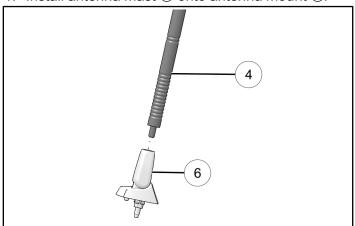
2. Seat antenna mount ⑥ in hood. Antenna mount will snap into place when fully seated.
