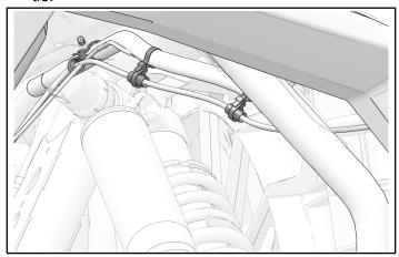
15. Route audio harness to front of vehicle along electrical chassis harness. Secure with two attached cable ties and one edge routing clip. Install GPS antenna 2A onto vehicle.
