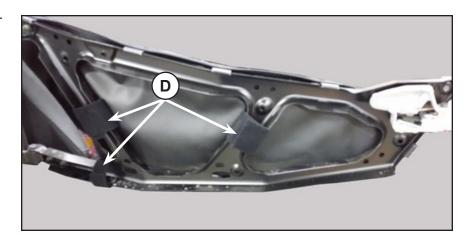
5. Reinstall the plastic door and attach six screws removed in the Step 1.
