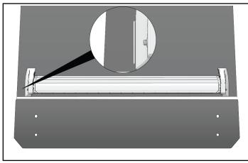
6. Align templates on markings made in previous step. Use tape to hold template in place. Verify distances (center of mounting hole to center of mounting hole) are correct, according to measurements below.
