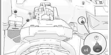
7. Open glove box lid and reinstall storage compartment. Install four retained dashboard fasteners around glove box opening.
