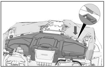
3. Ensure that both rubber boots are properly seated around hood panels. Only upper lip should be visible, as shown with inset.
