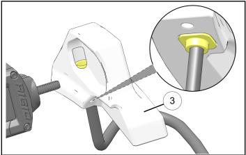
3. Loosely install left light bar mount ③ to light bar with one washer ⑦ and nut ④.
