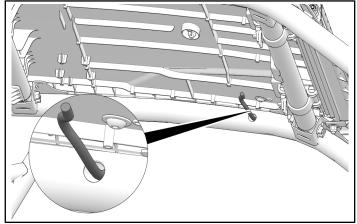
4. Slide grommet (18) onto light bar harness (1). Tape light bar harness (1) to fish tape and pull back through hole and out opening in lower brace. Once wire is routed, install grommet (18) into round opening in ROPS to seal.
