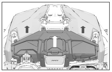
Ensure that tabs on panels are aligned in slots on dashboard top. (Passenger-side panel shown; driver-side panel similar.)
