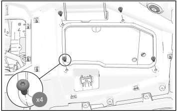
8. Install front of dashboard with three retained dashboard fasteners.
