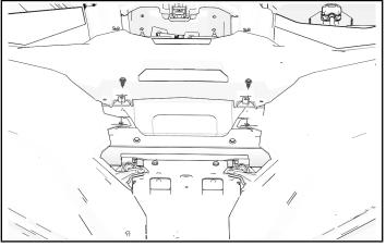
6. Tilt steering wheel down. Install four retained screws through dashboard top and torque to specification.
