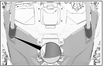
4. Reinstall two retained front dashboard fasteners into front edge of top dashboard.
