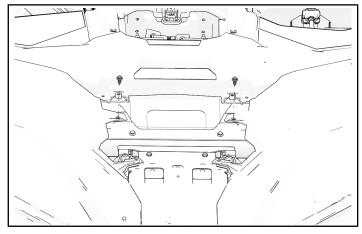
7. Carefully lift edge of left front hood panel to release tab from dashboard top as shown.
