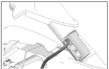
3. Locate fish tape and pull from round opening in roll cage as shown.
