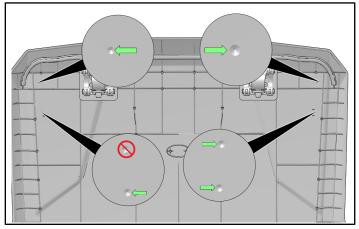
2. Drill four holes in outermost dimples as shown.
