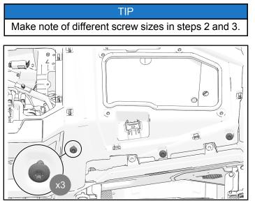
4. Tilt steering wheel down. Remove and retain four dashboard fasteners from dashboard surrounding steering wheel.
