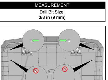
3. Drill one hole in driver side middle hole as shown.
