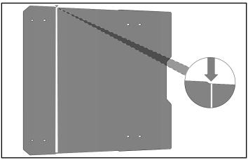
5. Center light bar assembly on roof. Align light bar along taped line. Mark roof along each outside edge of mounting brackets.
