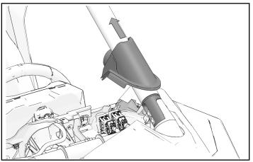
2. Feed fish tape (or equivalent) into opening in lower roll cage brace and up tubing, toward roof.
