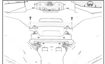
6. Remove and retain two push-pin rivets from front side hood panels.
