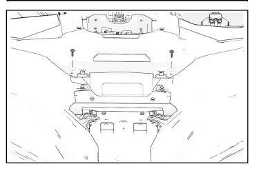
5. Install hood panels to with two retained push-pin rivets
