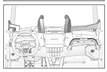
2. Open glove box lid. Remove and retain four dashboard fasteners around glove box opening.
