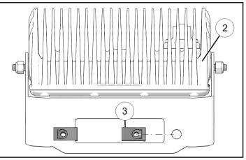
3. Connect lightbar harness connector 1A to lightbar assembly (2).
