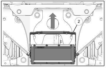
5. Install fascia lightbar to bumper assembly with two fasteners ④, passing through fascia, bumper, and into lightbar mounting bracket.
