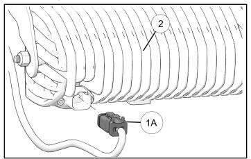
4. Align light bar assembly (2) with underside of bumper assembly.
