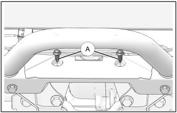
Install two U-clips (3) onto lightbar assembly (2) mounting locations.
