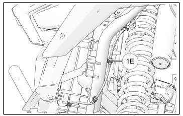
Route lightbar harness ① to right side of vehicle. Secure to chassis electrical harness with three cable ties ⑤ (not shown) at taped locations 1F.
