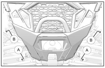
2. Remove bumper fascia from vehicle and carefully set aside.
