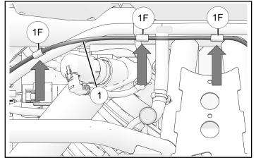
9. Route lightbar harness ① through entry in firewall and into under-dashboard.
