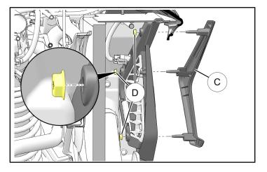
c. Install front LH accent light ① to fascia using three retained nuts ①.
