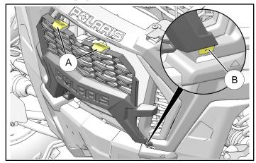
b. Remove LH trim © from front fascia by removing three stamped nuts ①. Retain nuts.
