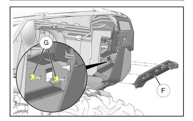
b. Install rear accent light ③ to fascia using four retained nuts ⑥.
