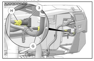
c. Remove cap from light connector (H), then plug into accent light.
