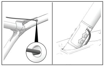
2. Tape roll-cage adapter harness ③ (end with bullet connectors) to fish tape and pull through lower roll-cage opening.
