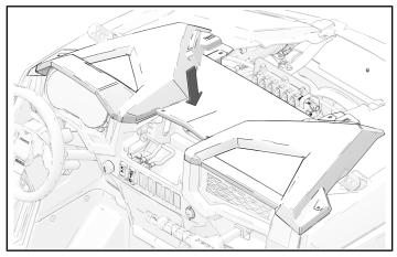
2. Install dashboard with four dashboard fasteners.
