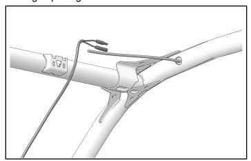
Leave enough excess harness to reach light bar (sold separately) and install attached grommet in roll-cage opening.
