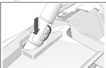
5. Install corresponding connectors. Wrap connections with electrical tape.
