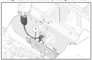
2. Install power connector to Polaris Pulse® bar.
