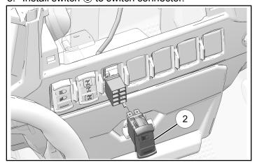
9. Install switch ② into dashboard and press until it snaps into place.
