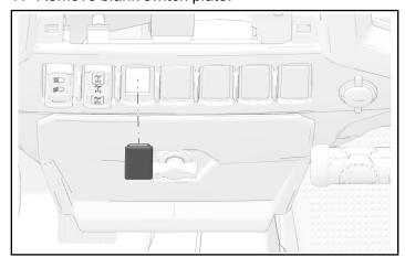
8. Install switch 2 to switch connector.
