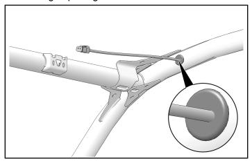
4. Put connectors, one-by-one, through small cutout in upper fender to reach dashboard harness.
