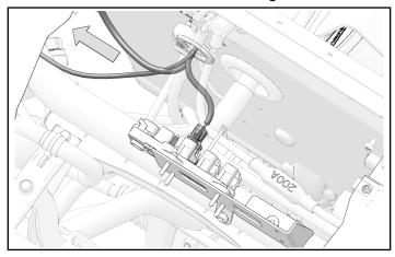
5. Put single switch connector through firewall grommet
