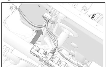
6. Pull switch connector through firewall grommet and pull towards front dashboard.
