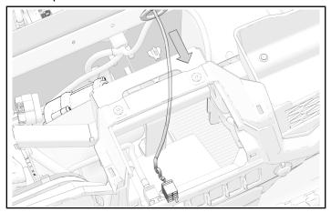
7. Remove blank switch plate.
