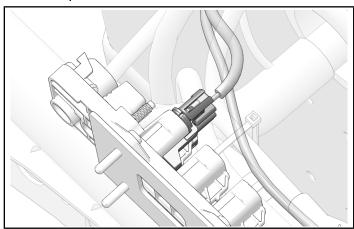
3. Install fuse relay onto firewall.
