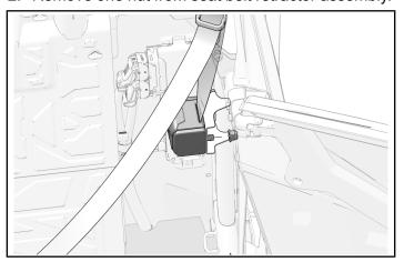
3. Remove one bolt and one nut from lower mount location.
