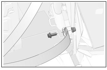
4. Remove one bolt and nut from upper mount location.
