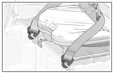
4. Secure seat belt hooks with one retaining pin (6) per hook.
