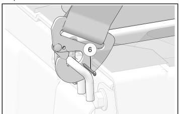
5. Position backrest assembly into seat base and lean back until headrest engages with receiver tube.
