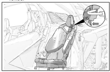
2. Remove one nut from seat belt retractor assembly.
