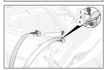
2. Rest harness on outside of each lower harness bracket and pass one fastener (4) through harness and lower harness bracket to install to nut.
