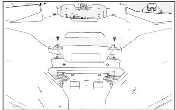
3. Tilt steering wheel down. Install four retained screws through dashboard top and torque to specification.
