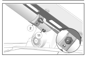
5. Lift windshield up and install strut <sup>(6)</sup> to ball-end of clamp assembly.
