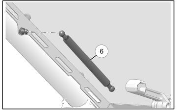
3. Assembly strut ball-end (1) onto clamp (2) with one fastener (1). Counter-hold ball-end and torque fastener to specification.
