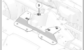
4. Torque four dashboard bracket fasteners  $\ensuremath{\overline{\textit{0}}}$  to specification.
