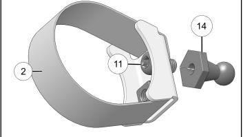
4. Wrap clamp (2) around A-pillar and position within inset of windshield frame. Loosely tighten clamp with one clamp fastener (1).
