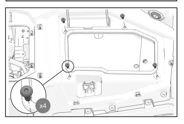
5. Install front of dashboard with three retained dashboard fasteners.
