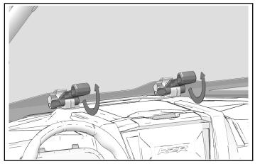
2. Rest latches on front latch snap position. Make sure latches snap into place.
