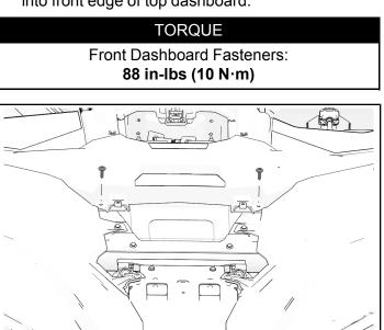
2. Install hood panels to with two retained push-pin rivets
