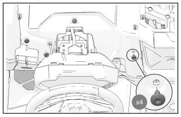
5. Remove and retain two dashboard fasteners from front of vehicle.
