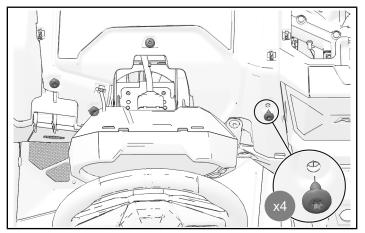
4. Open glove box lid and reinstall storage compartment. Install four retained dashboard fasteners around glove box opening.
