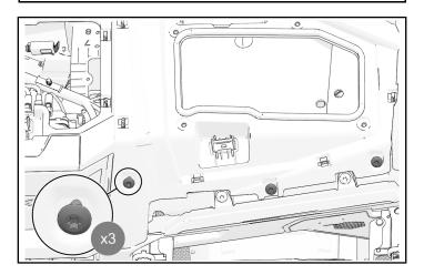
4. Tilt steering wheel down. Remove and retain four dashboard fasteners from dashboard surrounding steering wheel.
