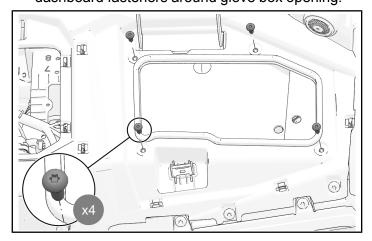
3. Remove and retain three front dashboard fasteners around glove box opening.
