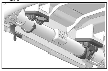
4. Install rear of roof panel with two roof fasteners ®.
