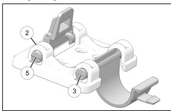
2. Test clamp hoop and clamp latch movement to make sure both are fully installed.
