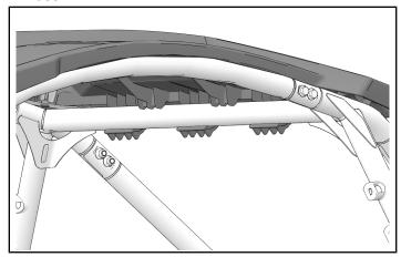
2. Rest clamp assemblies onto front ROPS crossbeam.
