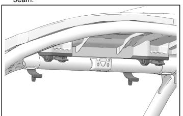
3. Wrap hoops around cross-beam and secure with latch.
