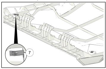
3. Windshield-equpped vehicles only: Install seal ⑥ onto front of roof panel.
