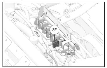
3. Install fuse relay to an empty port on the firewall.
