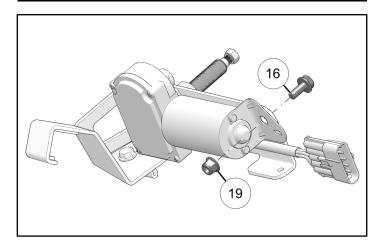
4. Tighten nut ② on motor assembly.
