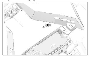
3. Install hose, coming from bottle, to hose fitting. Use one cable tie ② to install hose to fitting.
