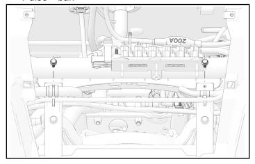
5. Install bottle assembly to chassis cross-beam with two fasteners (5). Torque two fasteners to specification.
