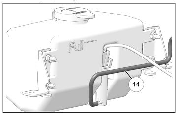
4. Remove and discard two fasteners from vehicle, located between chassis harness and Polaris Pulse ® bar.
