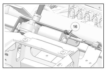
7. Install windshield wiper harness connector **5F** to motor.
