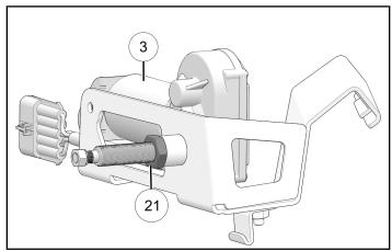
3. Install motor to motor mount with one fastener (16) and one nut (19). Counter-hold nut and torque fastener to specification.
