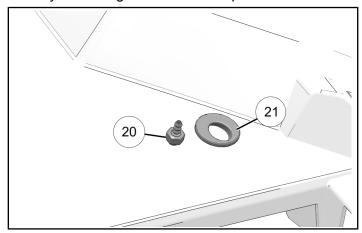
2. Put dashboard on vehicle so that motor shaft passes through grommet.
