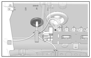
5. Pull harness through grommet and put switch connectors near empty switch plates.
