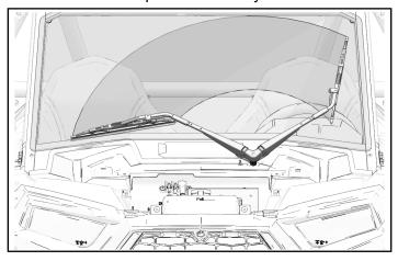
5. Install wiper arm with one nut and one washer, retained from *Step 1*.
