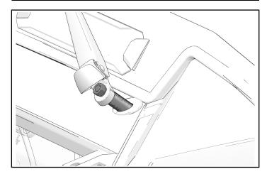
6. Install windshield wiper hose to dashboard hose fitting with one cable tie ③.
