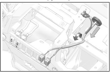
6. Remove and discard two switch plates from dashboard.
