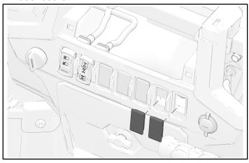
7. Install two switches ® and 9 to switch connectors **8F**.
