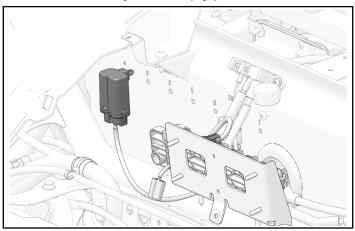
4. Put remaining switch connectors and motor connector through firewall grommet.
