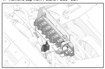
2. Install power connector **3F** to Polaris Pulse® bar.
