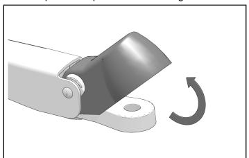
4. Place wiper arm onto wiper arm shaft in a position that will allow wiper blade to fully clean windshield.
