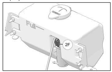
3. Install washer fluid hose (4) to the bottom of the washer fluid pump. Use one cable tie (3) to install hose to pump fitting.
