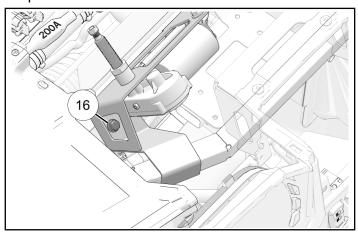
6. Install right side of mount with one fastener (6). Torque both fasteners to specification.
