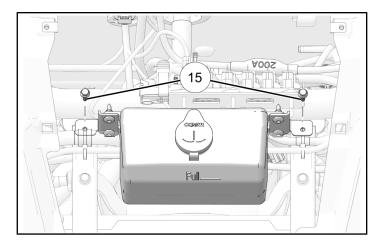
6. Counter-hold nuts on bottle bracket and torque fasteners to specification.
