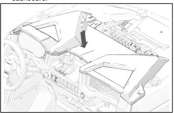
2. Install dashboard with four dashboard fasteners.
