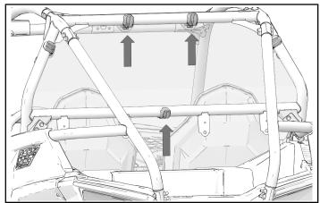
4. Apply pressure to outside of Lock & Ride<sup>®</sup> clamps to install onto roll-cage.
