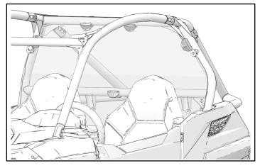
3. Move rear panel upwards until Lock & Ride<sup>®</sup> clamps are on horizontal tubes.
