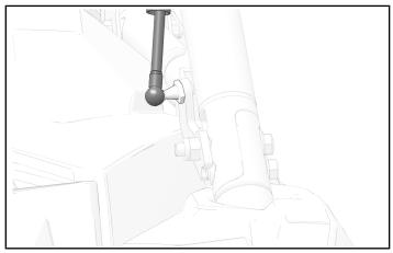
5. Counter-hold nuts and torque two top mounting fasteners ② to specification.
