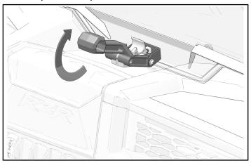
2. Rest latch handle on front latch snap position. Make sure latch handle snaps into place.
