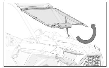
4. Install strut onto strut bracket ball-end.
