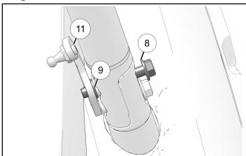
5. Install strut bracket ① with one nut ②. Counterhold nut and torque fastener to specification.
