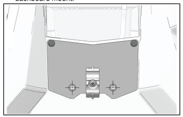
4. Remove dashboard mount. Drill two **5/16 in (8 mm)** holes in dashboard.
