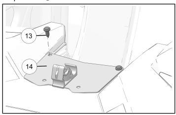
3. Mark dashboard to drill two holes. Remove dashboard mount.
