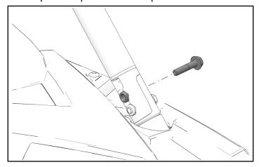
2. Partially install one fastener ® into retained nut.
