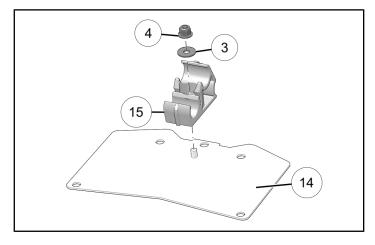
2. Install rear of dashboard mount (4) with two pushpin rivets (3).
