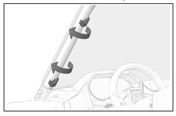
Windshield may need repositioning. If needed, release top clamps and slide windshield up along ROPS.
