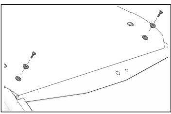
3. Slide two windshield clamps ② onto windshield frame. With clamps ② tightly wrapped around ROPS, secure to windshield frame with two flange sleeves ⑥ and two fasteners ④.
