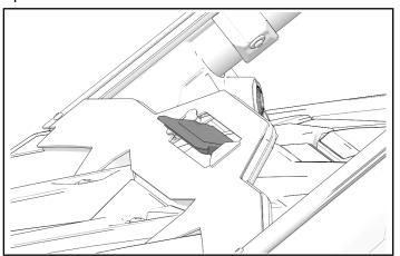
To restrict airflow through the vent, from inside the vehicle push on the top of the vent flap until it closes.
