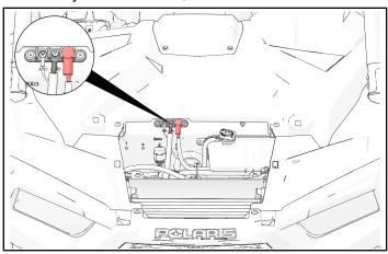
7. Route loose ends of cables ⑤ and ⑥ upward, then connect ring terminals to terminal block. Install terminal block post nuts finger tight only. Additional connections will be made in next step.
