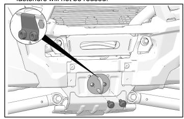
2. Install winch backer plate ® to underside of support channel using nut ①. Align holes in plate and channel, then hand-tighten nut.
