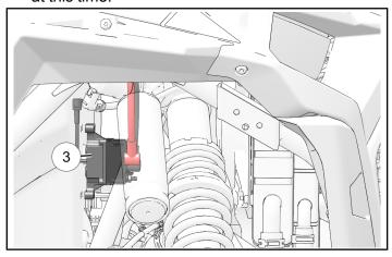
3. Route winch cables behind suspension and towards contactor.
