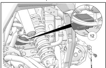
2. Join connector 16B on Y-splitter harness (6) to connector 12C on wireless receiver 12.
