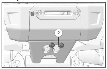
7. Torque four fasteners ② to specification.
