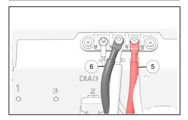
8. Route two ring terminals 1H and 1J rearward and upward, then connect to terminal block. Install terminal block post nuts finger tight only. Additional connections will be made later.
