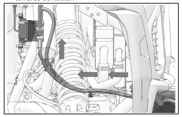
Connect winch ring terminals 1A and 1B to posts on contactor ③. Ensure final cable routing (with contactor installed to firewall) will prevent contact with hot components, sharp edges, or moving parts.
