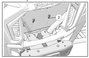
6. Install lower end of winch assembly to vehicle using two winch fasteners ②.
