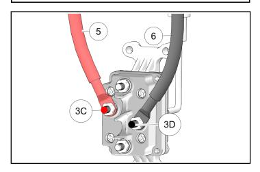
2. Position contactor ③ near firewall in approximate location shown. Do not install contactor to firewall at this time.
