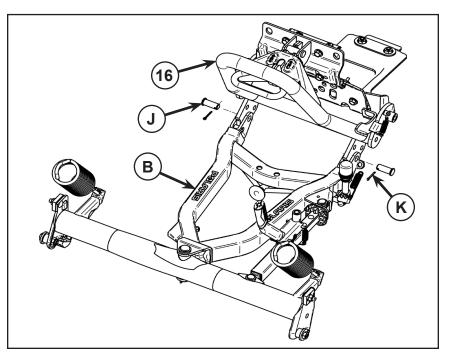
**NOTE:** Make sure the hook up (16) can move as shown in the picture. If this is not the case, remove the clevis pins (2) and reposition the handle so that the stoppers allow the part to move in the right angle.
