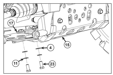
**NOTE**: M6-1.0 x 30mm hex flange bolts have been provided with this kit and should replace the two lower fascia bolts to account for the extra thickness added by the mount plate. See figure for proper bolt placement.
