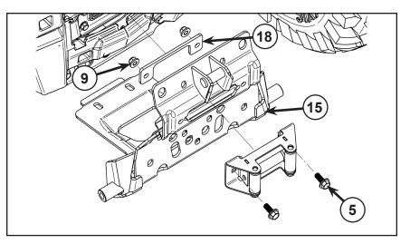
B. Fasten the winch 4500 lbs fairlead to front of mount plate (15) using the two M10-1.5 X 30 mm hex flange bolts (5), two M10-1.5 flange nylon nuts (9). Torque to 40 ft. lbs. (54 Nm).
