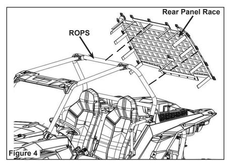
Place the rear panel race (PN 2635080) onto the vehicle body. Drill the holes at five locations to install the rivets. Figure 5.
