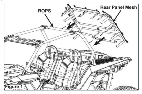
Place the rear panel mesh (PN 2635219) onto the vehicle body. Drill the holes at five locations to install the snaps. Figure 2.
