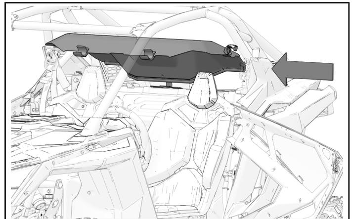
4. Carefully, position rear panel so that side clamps rest on vertical ROPS.
