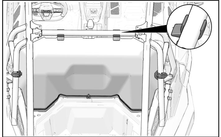
5. Compress seal to fit securely against body panel. Ensure mounting bracket is outside of rear panel.
