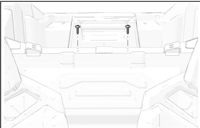
2. Install rear panel bracket (2) with two retained fasteners. Ensure vertical part of bracket is facing rearward.
