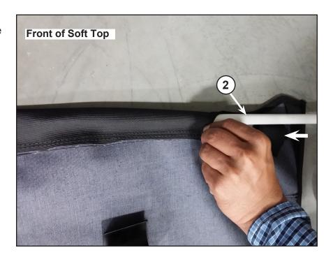
3. Insert the one end of front rod (2) into the webbing pocket as shown in figure.
