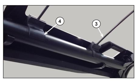
6. Press and fit two clamps (4) at the rear ROPS bar. Insert the other ends of support rods (3) into the holes of the rear clamps by bending the rods slightly as shown in figure.
