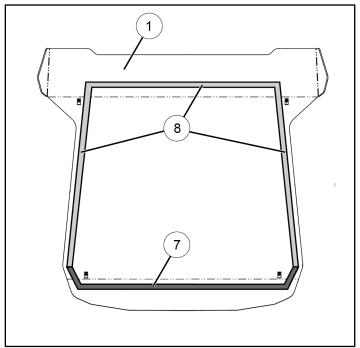
c. Peel adhesive backing from 10 mm foam tape ®, then apply tape to SIDE and REAR edges of roof panel ① as shown, trimming as required. Press tape firmly into place.
