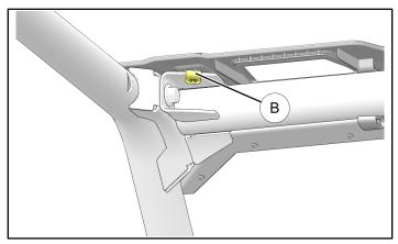
3. Install two clip nuts ⑤ to rear ROPS crossmember, upper OUTBOARD gussets. Upper inboard gussets will not be used.
