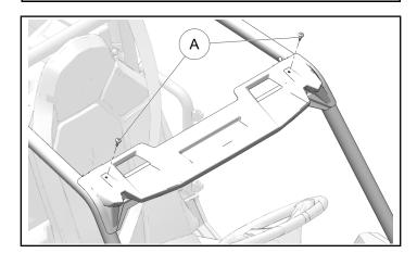
2. OPTIONAL: Replace two clip nuts ® on forward ROPS cross-member, upper rear gussets, with new clip nuts ⑤.
