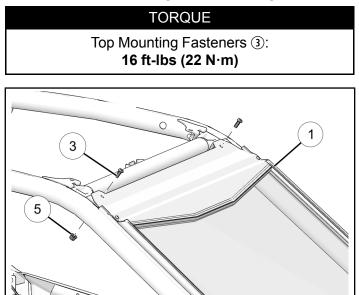
Aluminum Roof-equipped vehicles: Use roof hardware for this mounting location. Ensure windshield mounting bracket is installed between roof and ROPS.
