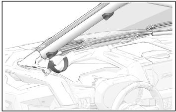
Windshield may need repositioning. If needed, release top clamps and slide windshield up along ROPS.
