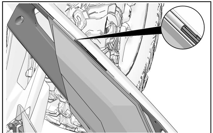
4. Hook bottom of door bag to bottom of door frame.
