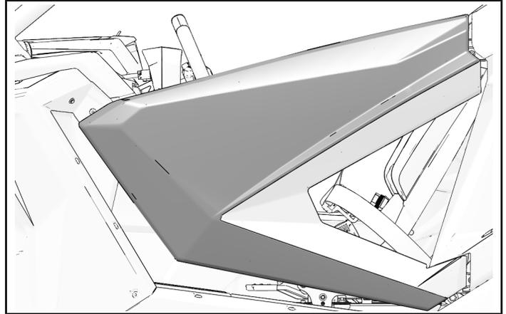
2. From inside of door, install door panel with eleven door panel fasteners.
