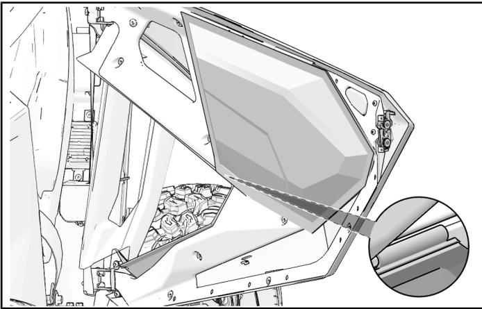
5. Wrap hook-and-loop fastener around door frame to secure front of bag.
