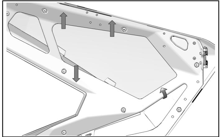
2. Align top of door bag with top of door structure.
