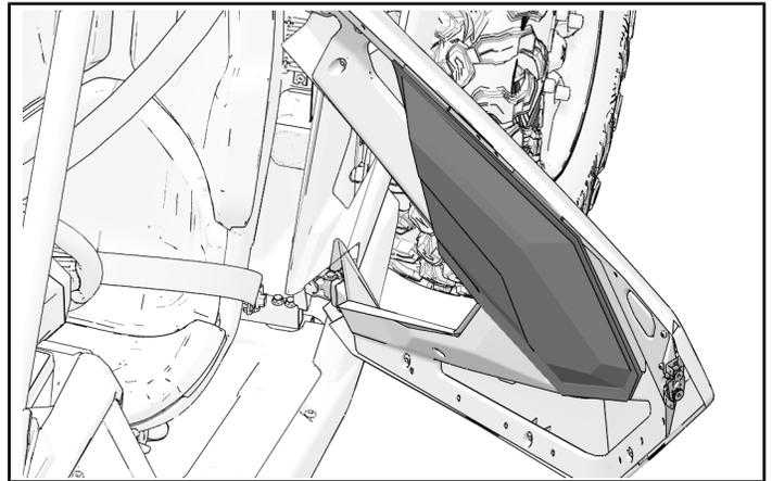
3. Carefully, but forcefully, pull back door panel and hook door bag onto door frame at two locations. Door bag hooks fit between door panel and door frame.
