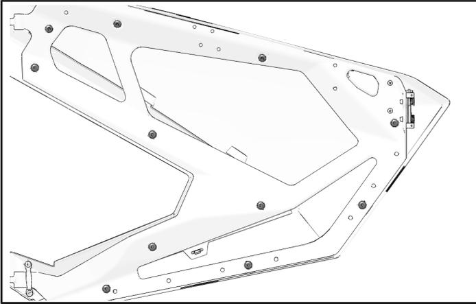
2. Remove door panel from door and carefully set aside.
