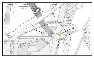
c. Route rear inboard harness clip (and driver safety interlock harness, if applicable) through new boot ⑤ and center console cutout, then install clip to vehicle mount bracket using bolt ③ and nut ④. Ensure proper orientation: harness clip is on FRONT side of mount bracket. Torque to specification.
