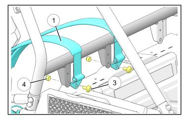
b. Install rear outboard harness clip to vehicle mount bracket using bolt ③ and nut ④. Ensure proper orientation: harness clip is on OUTBOARD side of mount bracket. Torque to specification.
