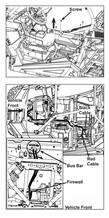
6. Detach the plastic plate by removing two screws (PN 7518980).
