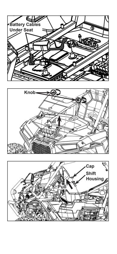
After removing shift lever cap and shift handle, take off the center console by removing the two screws (PN 7519650) and the four tuff lock rivets (PN 7661855).
