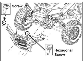
8. Mount the winch plate onto the vehicle with four screws (PN 7519372) and lock nuts (PN 7547423).
