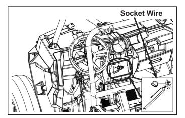
19. Feed the socket wires from inside of cab through the grommet in the firewall.
