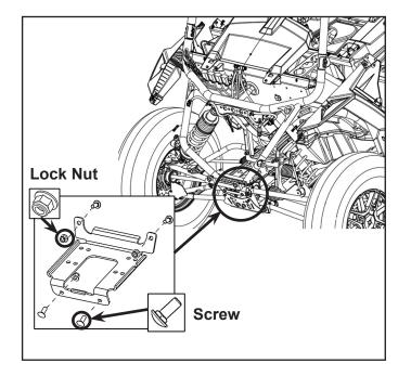
7. Take off the front fascia by removing six hexagonal screws (PN 7518529) and four screws
