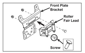
13. Front Plate Bracket installation:
