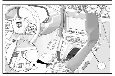
3. Attach console trim ① to upper center console using two push pin rivets ⑧.
