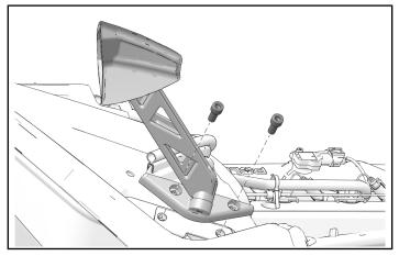
2. Torque mounting screws to specification.
