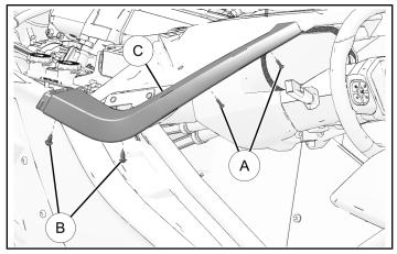
2. Torque two screws to specification.
