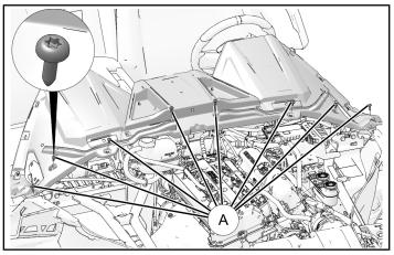
3. Torque eight screws to specification.
