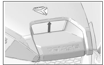
4. Pull hood upward and forward, rotating hood to a vertical position.
