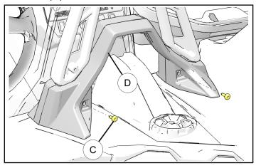
5. Remove lower roll hoop covers (B) and (D) around the roll hoop (E).
