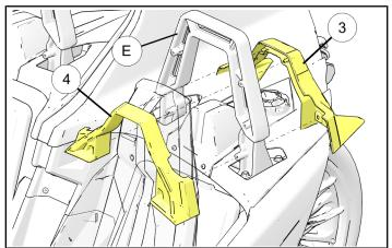
2. Ensure two lower roller hoop cover ③ and ④ halves are aligned to each other as well as screw holes are aligned with roll hoop (E).
