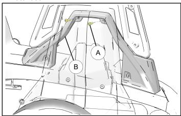
3. Using T40 Torx® drive remove two screws (C) located at the lower front of the lower roll hoop cover (B). Retain screws for later use.
