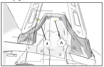
4. Using T40 Torx® install two retained screws (C) at the bottom of lower roll hoop cover ④. Do not fully tighten.
