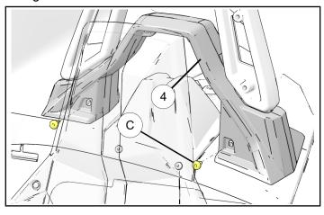
5. Using T40 Torx® install two retained screws (C) at the bottom of lower roll hoop cover ③. Do not fully tighten.
