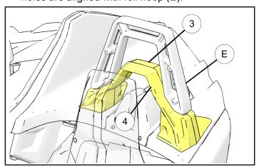
3. Using T25 Torx® install two retained screws (A) at the top of lower roll hoop covers ③ and ④. Do not fully tighten.
