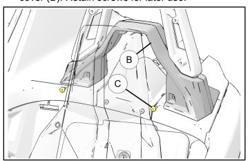
4. Using T40 Torx® drive remove two screws (C) located at the lower back of the lower roll hoop cover (D). Retain screws for later use.
