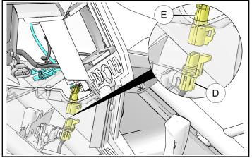
Connect infotainment harness connector E to garage door opener harness connector F. Connect electrical harness connector D to garage door opener harness connector G.
