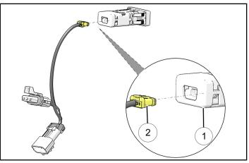
3. Route garage door opener harness through opening created in **Step 1** before installing garage door opener module ① in same opening.
