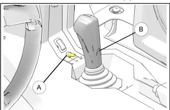
3. Firmly pull up on shift knob (B) to remove from transmission shift rod adapter as shown.
