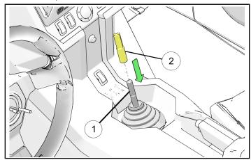
4. Place shift knob cap (G) onto transmission shift adapter ①.
