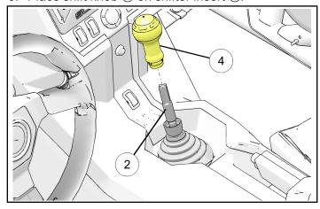
Using 2.5mm hex wrench, install three set screws
