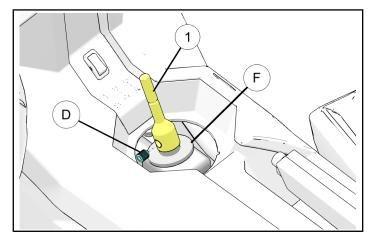
2. Install new rubber boot ③ around transmission shift rod (F). Ensure edges are properly seated.
