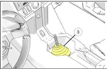
3. Slide shifter insert ② onto the transmission shift rod adapter ①.
