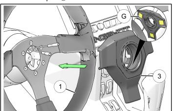
b. Align horn pad ③ on steering wheel ① and firmly press down.
