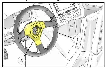
5. Locate horn wires in center of steering wheel assembly ①. Connect horn wire tabs to horn button and install horn button ② by firmly pushing around its edges.
