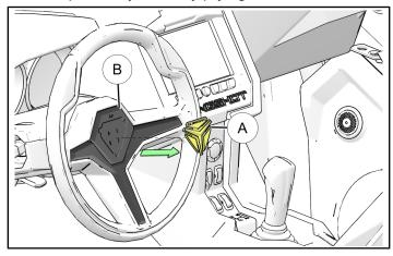
2. Remove and discard horn pad ® from steering wheel © by prying up from bottom of horn pad ® and working upwards until all three arms of horn pad ® are removed.
