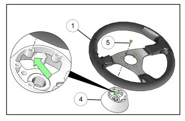
2. Place horn wires **(F)** through opening of hub adapter while aligning steering wheel assembly **(1)** onto steering wheel shaft **(E)**. Left and right steering wheel spokes should be horizontal while third spoke should be directed downward.
