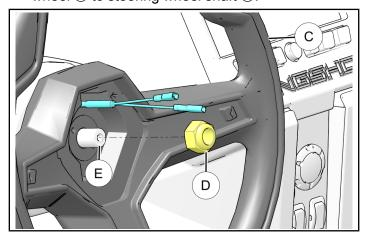
4. Mark top center of steering wheel shaft to aid in Performance Steering Wheel alignment.
