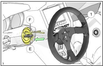
Align steering wheel assembly ① with mark made in Step 4 of Stock Steering Wheel Removal.
