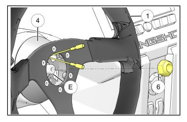
4. Clean steering wheel spoke surface with solvent wipe prior to installing horn pad.
