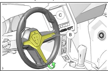
3. Remove and discard nut ① securing steering wheel ① to steering wheel shaft ①.
