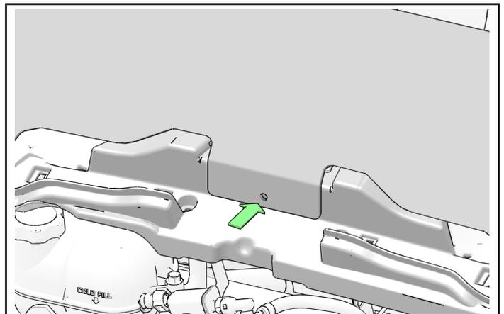
6. Reinstall windshield ① by engaging tab and slot in the front and aligning three holes on windshield. Install screw ③ and washer ④ onto the windshield. Torque screws to specifications.
