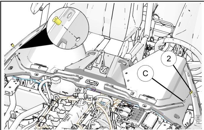
4. Install tinted windshield (1) by first engaging the tab and slot in the front then aligning the mounting holes on windshield and main visor.
