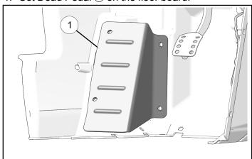
2. Mark the four holes. Drill the marked holes, keeping the drill perpendicular to the floor board surface.
