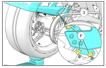
3. Thread three nuts (9) on three retained bolts (F) **Do** not tighten at this time.
